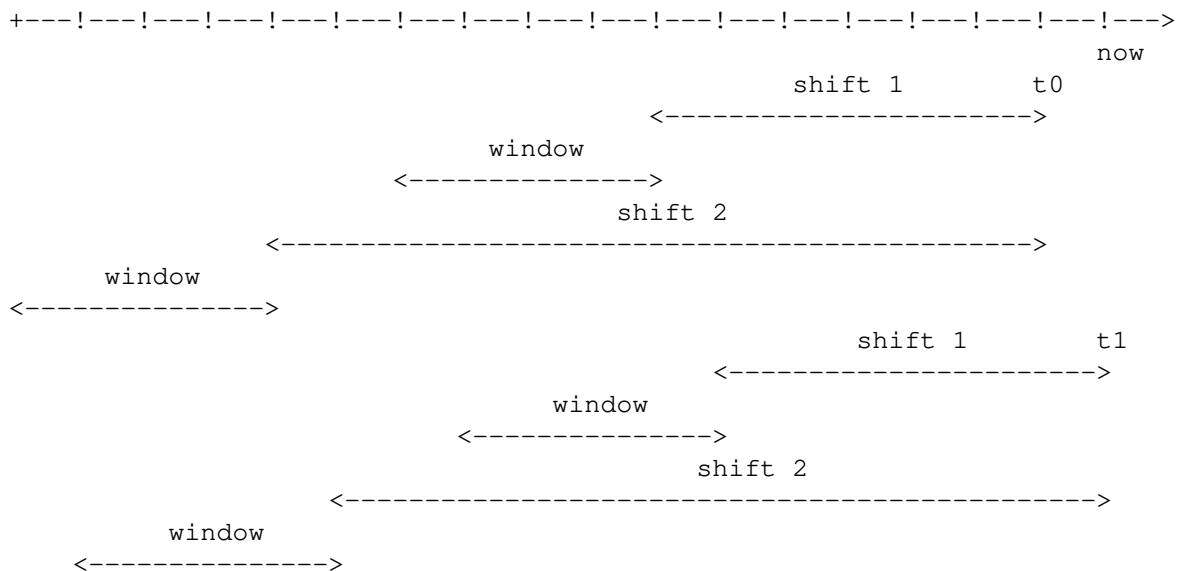
Value at sample (t0) will be the average between (t0-shift1-window) and (t0-shift2-window)
